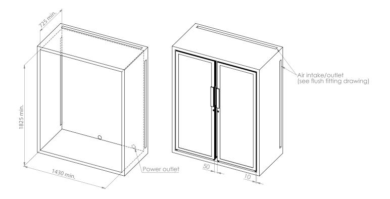
Please note: If installing two cabinets side by side, they must be separate by at least 5cm. This allows adequate circulation of air around the cabinets, ensuring that they function correctly.
