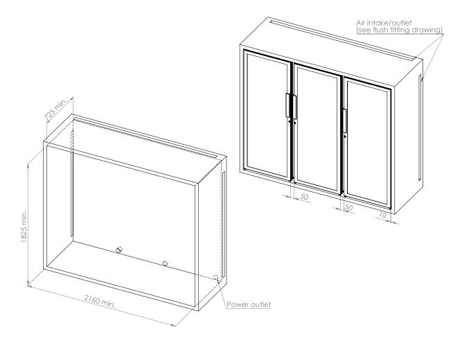
Please note: If installing three cabinets side by side, they must be separate by at least 5cm. This allows adequate circulation of air around the cabinets, ensuring that they function correctly.
